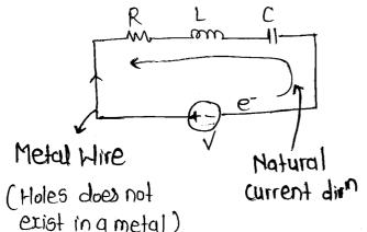
Conventionally, ---> the current direction is taken in the direction of the positive charge moment.
